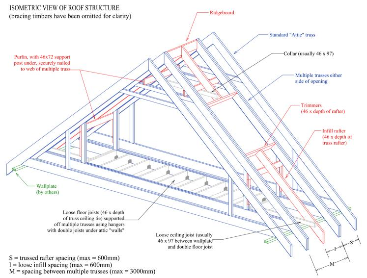
The approximate number of plys of the multiple trusses may be determined from the following table:
