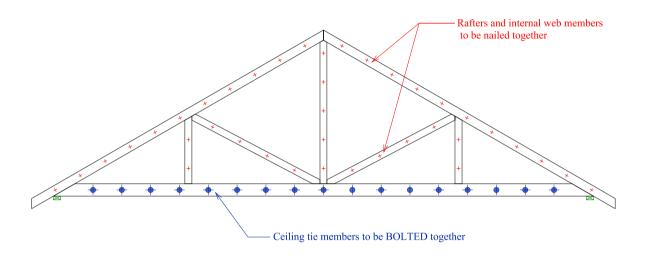
Unless stated otherwise on drawings supplied with the trusses, all nails / bolts are to be fixed on the centreline of the members and be spaced at 400mm centres.
