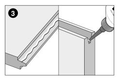
Apply Kronobuild<sup>®</sup> D4 Adhesive along the full length of both the tongue and groove profile as boards are fitted. The joints should be securely bonded when the boards are interlocked.
