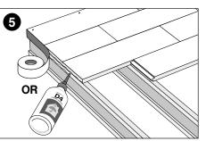
Use Kronobuild<sup>®</sup> specially formulated D4 Adhesive or Kronobuild<sup>®</sup> reinforced weather resistant tape to seal cut edges, perimeter edges, stairwells and mechanical fixing heads.
