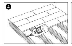
Repeat the application steps on subsequent rows of boards which should be laid in a staggered pattern. Short end joints, including perimeter edges, must fall on a secured joist or noggin. (See reverse for mechanical fixing pattern). Any excess adhesive should be left to dry then removed. If in doubt consult NHBC guidelines.
