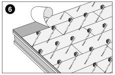
For Kronobuild<sup>®</sup> Fast Protect and Kronobuild<sup>®</sup> Fast Clean. Once the construction is completed, weatherproofed and all decorating work is finished the flooring can be cleaned simply by peeling back the protective film slowly and steadily from the shortest edge.
