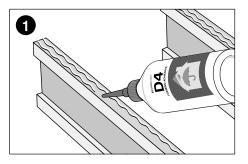
Using Kronobuild<sup>®</sup> specially formulated D4 Adhesive lay two 6mm beads to the top of the joist the first boards are to be fitted to.
